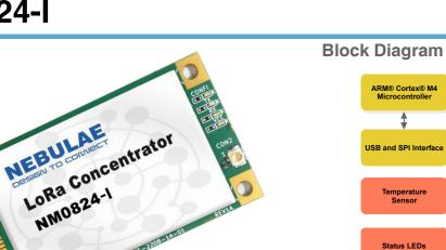
NM0824-I is SX1302 based compact size, Low power LoRa concentrator board with 2 x SX1250 & 1 x SX1261 radio with onboard I2C based Temperature sensor. Compared to SX1301 LoRa<sup>®</sup> chip, it offers higher sensitivity, less power consumption, and lower operating temperature.
