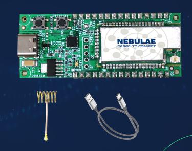
Arduino EVK or Evaluation Kit featuring LoRa® technology is designed to facilitate beginners, developers, and students to learn LoRa and IoT technology quickly. It helps users, turn their idea or Proofs-of-Concept into practical applications and make the IoT a reality. It is easy to program, create and connect your things everywhere.
