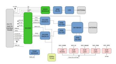
NLN0821-I is SX1303 based compact size, Low power LoRa concentrator board with 2 x SX1250 radio with onboard GPS and I2C based on-board Temperature sensor. Compared to SX1301 LoRa<sup>®</sup> chip, it offers higher sensitivity, less power consumption, and lower operating temperature.
